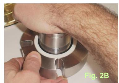
**Ensure** that all pins are fully and equally engaged into holes visually (**Fig.2C**). As a final check, try to pull rotor off from sleeve by hand. If rotor moves off from sleeve, pins were not fully locked in. **Visually** check pins, rotor and sleeve. If parts are ok, retry step 2. If unsure, please consult with factory.
