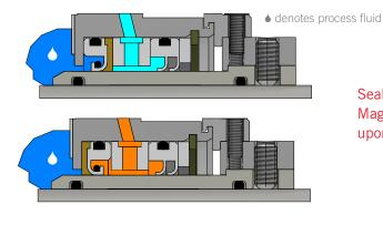
Seals can be grease packed with Magnalube®-G or Molykote™111 upon request.
