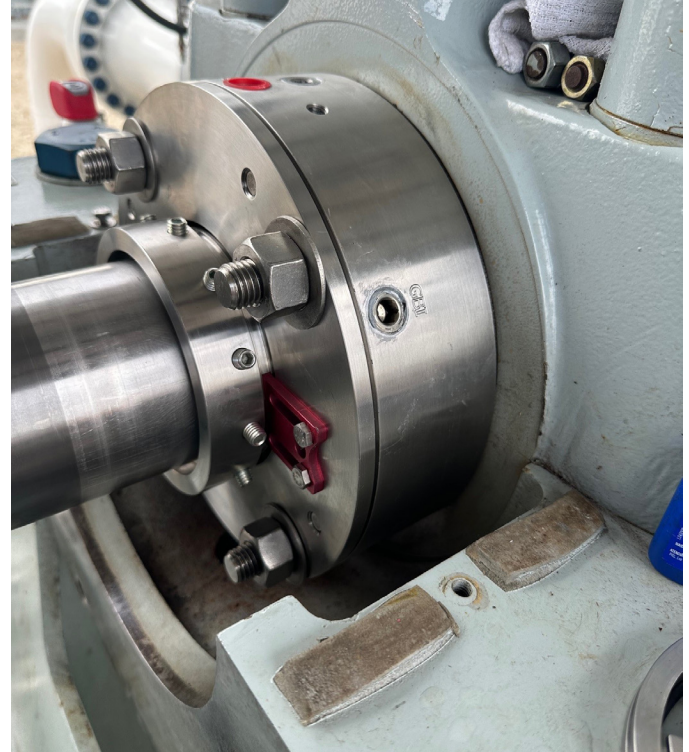
Figure 6. Flexaseal HPSS/CPH Seal Fitted to the Equipment
